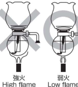
△ If heating over a gas stove, use a low flame to avoid heating the stand and other part of glass.
