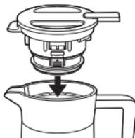
Push the inner stopper straight down. Push firmly until you hear a click. If the inner stopper is not securely set, the drink may leak.
