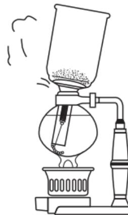
If the water is boiling too fast (is too hot), remove the flame (move burner and holder) to reduce the temperature. Attach the upper bowl only after bubbling has calmed, and then reheat. (You can also tilt the upper bowl so that the chain attached to the filter causes tiny bubbles to be produced.)
